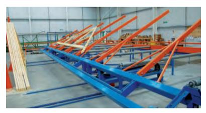
The Truss Stacker moves the truss Horizontally on powered rollers and Automatically lifts it to a vertical position creating a stack of trusses with no operator required.
